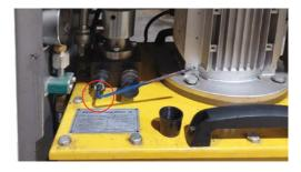
Momentarily bring the unit up to pressure by feeding V former against the mandrel. Adjustments are small. Half a turn to a turn max should be all that is required. Turning counter clockwise will reduce pressure. Adjust to 4000 PSI/28 MPa.
